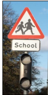
Wig-wag lights can be mounted below the sign assembly or at the side usually as part of a backing board.
